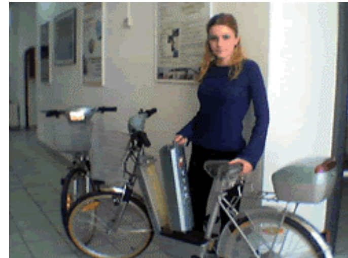
PICTURE 4-4: The battery is removable and can be recharged using a common household socket
