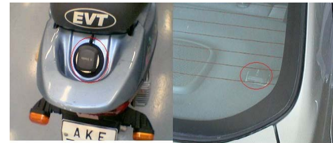
PICTURE 6-4: GPS antennas at the electrical shooter and Toyota Prius
