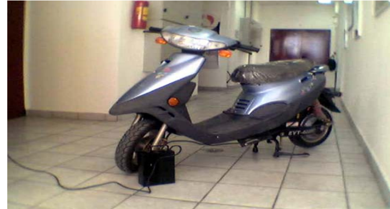
PICTURE 4-6: Electric scooter during recharging. The electric motor can be seen on the left hand side of the picture.
