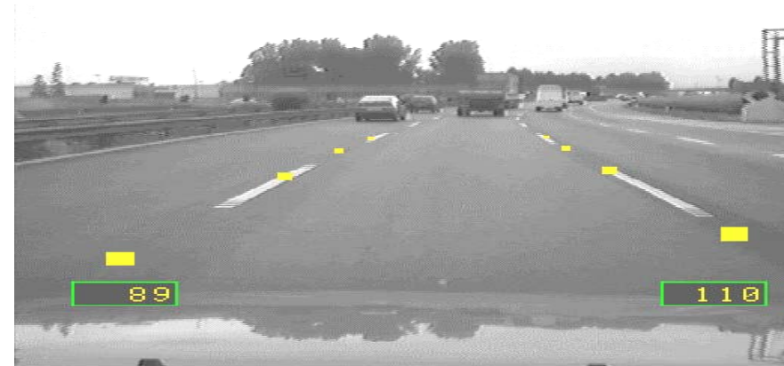
PICTURE 6-2: Lane switching monitoring system
